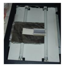
We lean the test and the shield on the bromograph glass. We expose the sector in the way and with the
